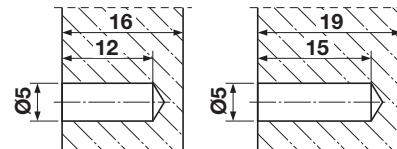
**Drill holes for the cabinet flap which comes in 2 parts
